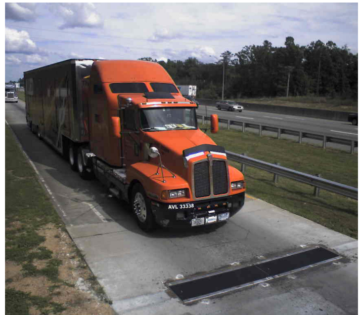
Truck passing through a Virtual Weigh Station using IRD-PAT Bending Plate™ WIM Scales (Single threshold weighing)
