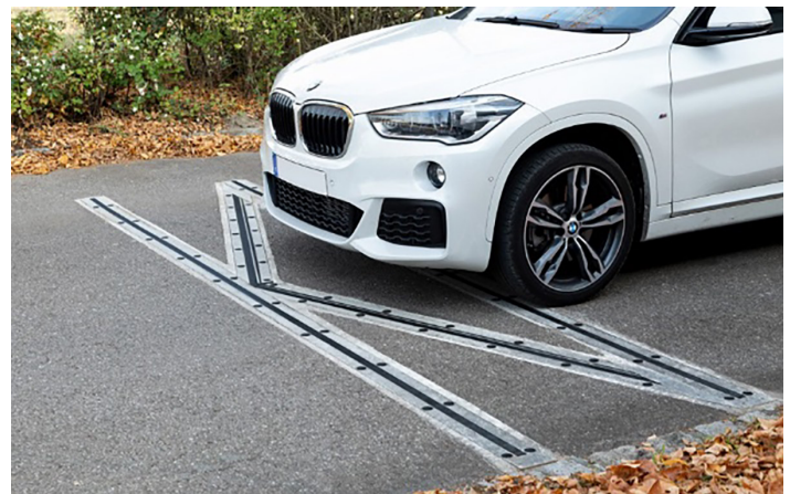
SL EZ sensor installation for axle-based classification
