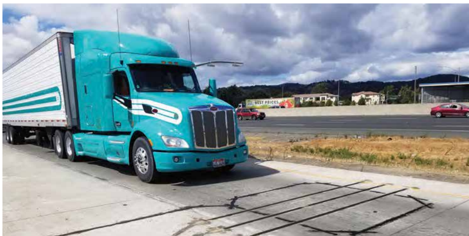
Tire safety screening in Cordelia, California, using TACS™
