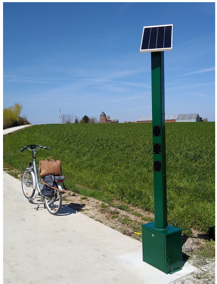
Solar-powered TOTEM TMA-3B3 bicycle counter
